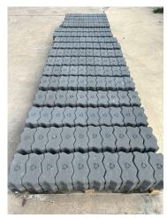
After improvement The Company repurposed the black sand by converting it into a raw material for producing "interlocking paving blocks", mixing it with cement at an optimal ratio. These paving blocks are now used for internal roads and walkways within the plant premises. This initiative significantly reduces the volume of waste requiring external disposal and supports the promotion of a circular economy.
