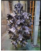
Before improvement: The jig used for shot blasting Carrier Differential parts could accommodate 12 pieces per cycle.
