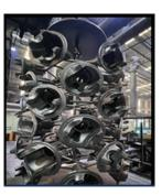
After improvement: The jig was redesigned to allow 36 pieces per cycle. This improvement significantly increases production capacity, leading to reduced processing time and energy consumption.
