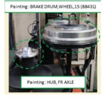
After improvement: Installed additional support pillar, enabling two parts to be painted per cycle. This increased production capacity, reducing both operational time and energy consumption.
